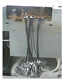
Fig: Wiring Harness connected to PCE
